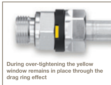
Yellow window completely visible after final assembly
