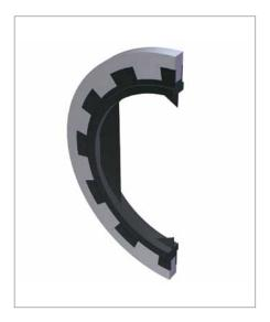
The Parker WT composite sealing washer consists of a metal washer and a rectangular elastomer sealing lip with an additional mechanical connection to the inside edge of the supporting washer. The serrations achieve a positive connection of the elastomer with the supporting washer and the phenomenon of sheared sealing lips which is frequently encountered with composite sealing washers is prevented.
