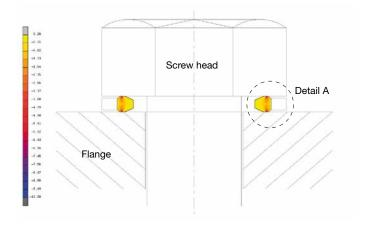
**Detail A: composite sealing washer**
