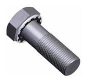
Parker WO series composite sealing washers are designed for radial sealing below the screw head in the area of the smooth (non-threaded) screw shaft. This provides three functionally relevant sealing areas. The elastomer sealing lip is chemically and mechanically connected to the metal carrier.
