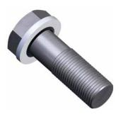
Parker WX series composite sealing washers have been designed to replace copper washers in high-pressure systems. The WX composite sealing washer is a time-tested and low-cost solution for screw head and flange sealing areas. The elastomer sealing lip is chemically bonded to the metal carrier.
