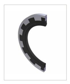
The Parker WO composite sealing washer consists of a metal washer and a circular elastomer sealing lip with an additional mechanical connection to the inside edge of the supporting washer. The serrations achieve a positive connection of the elastomer with the supporting washer and the phenomenon of sheared sealing lips which is frequently encountered with composite sealing washers is prevented.
