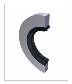
The Parker WZ composite sealing washer consists of a metal washer with a rectangular cross-section and an elastomer sealing lip with a trapezoidal cross-section that is vulcanised to the inside. It is a further development of the WX series and has an additional self-centring function.
