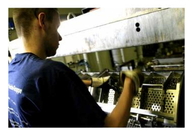
Bare metal surfaces must be protected against corrosion and prepared for the elastomer vulcanisation. Typically, the metal surface is corrosively closed by a passivation technique and prepared for the subsequent vulcanisation of the elastomer sealing lip by means of a special phosphate coating.
