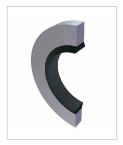
The Parker WX composite sealing washer consists of a metal washer with a rectangular cross-section and an elastomer sealing lip with a trapezoidal cross-section that is vulcanised to the inside.
